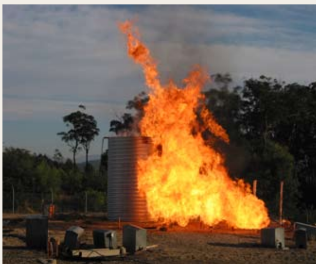
▲ ABOVE AND TOP RIGHT: RAINWATER TANKS WERE TESTED UNDER SIMULATED BUSH-FIRE CONDITIONS AT THE RFS TEST FACILITY AT MOGO.
